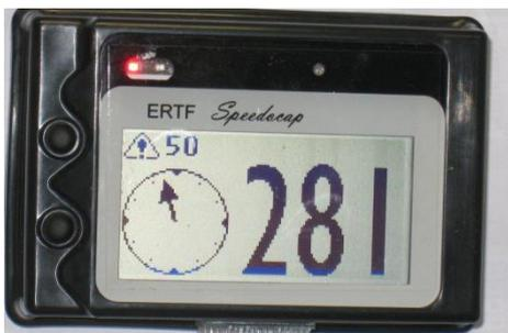
Here the red led is active because the driver is over the limit defined by the Speedox function. If the lamp is connected, it will also be on.
